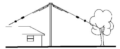
**DX-A -** 160-80-40 Meter 1/4-wave Twin Sloper - A top low frequency DX antenna. Combines the tremendous DX firepower of the 1/4-wave sloper with the wide bandwidth of the 1/2-wave dipole. One leg is 67 ft., the other 55 ft. Installs like an Inverted-V with ground return accomplished thru tower or down-lead.
