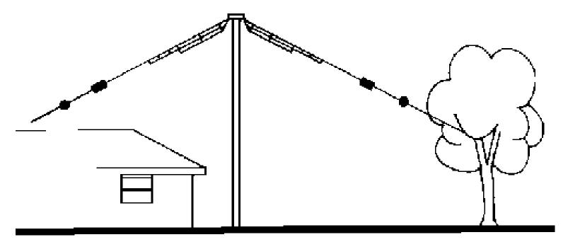
**DX-A** - 160-80-40 Meter 1/4-wave Twin Sloper - A top low frequency DX antenna. Combines the tremendous DX firepower of the 1/4-wave sloper with the wide bandwidth of the 1/2-wave dipole. One leg is 67 ft., the other 55 ft. Installs like an Inverted-V with ground return accomplished thru tower or down-lead.
