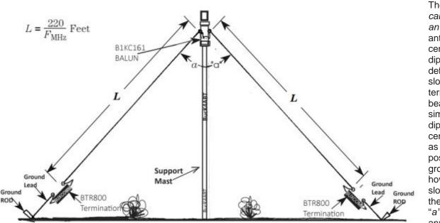
The vee- beam can be viewed as an inverted dipole antenna fed in the center like a dipole. By the definition, the sloping, terminated, veebeam, has a similarity to the dipole. The center is elevated as high as possible from ground surface, however, the ends slope to close to the surface. Angle "a" can be almost anything, provided
