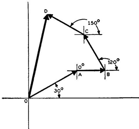
vector diagram for their addition is illustrated in Fig. 6-8, where the vectors are all drawn to a scale of 1 inch equal to 10 volts. Vector OA is first drawn at a phase angle of 30 degrees with its initial point starting at the origin of the main coordinate system. Then the tail of vector AB is drawn from the head of vector OA at an angle of zero degrees from point A. Then from the head of vector AB the tail of
